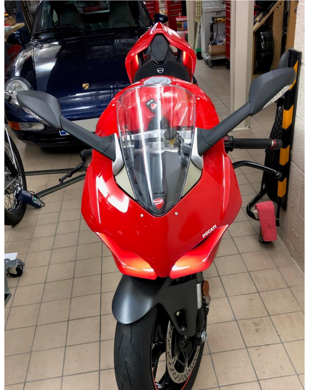
Ducati 2019 Panigale V4 after converted to folding rear view mirrors per Ducati 2012 1199 Panigale.
