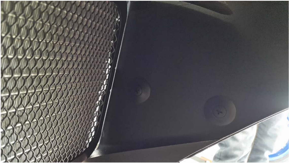
Plastic rivets seen from the inside
